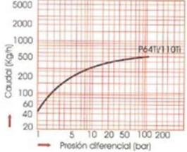
Capacities given are continuous discharge capacities of hot condensate. The cold water capacity at start-up condition will be 2.5 of the hot condensate capacity.
